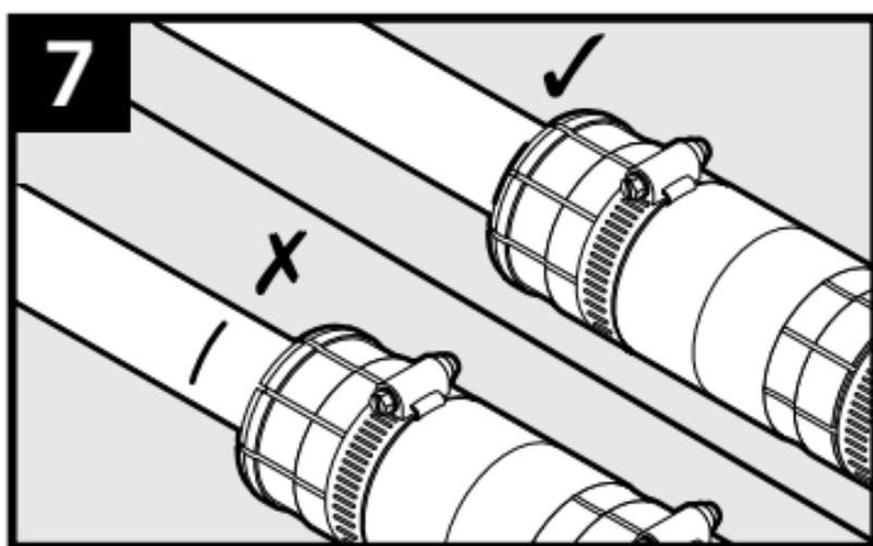
Once duct ends are aligned, use the markings made in Step 2 to reposition the coupler centrally over the duct splice.
