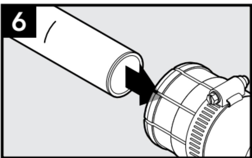
Push conduit into coupler. To allow duct ends to align in tight spaces, coupler can be pushed completely on to one duct.
