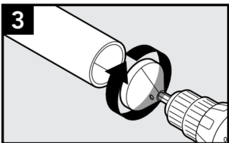
Chamfer the end to allow for smooth insertion.
