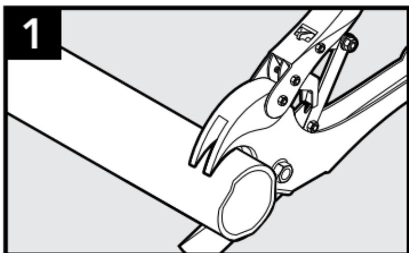
Cut conduit flush with duct cutters.
