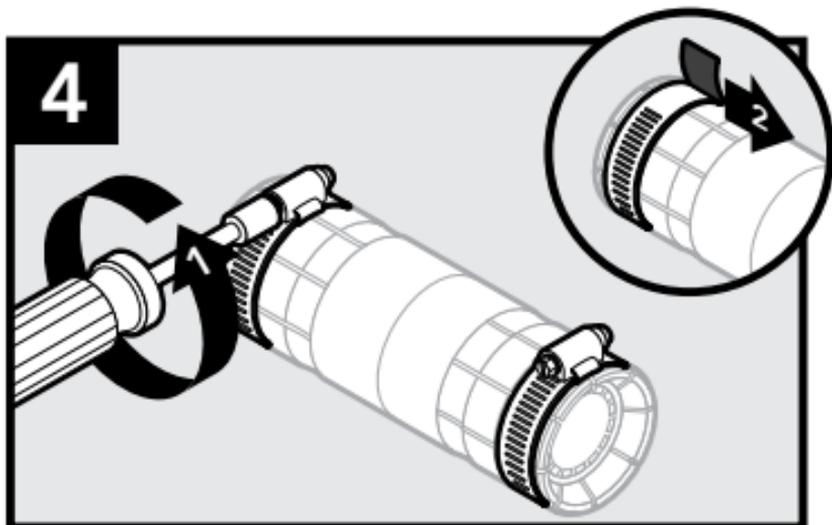
Loosen band clamps and move them towards the middle of the coupler. Lightly tighten to hold in place during conduit insertion.
