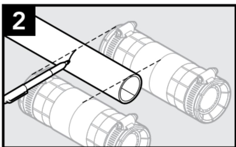
Align both ducts at the center of the coupler and mark ends.
