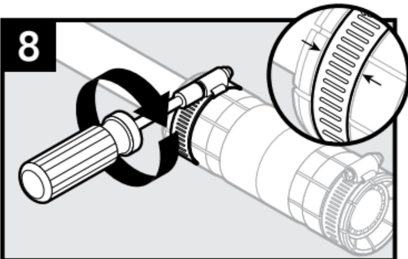
Verify the band clamp is positioned in the groove and fully tighten it down with a 5/16" nut driver. Never use a drill to tighten clamp.
