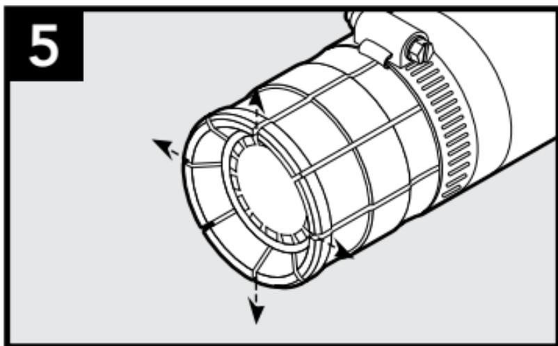
Spread tabs on each end of the coupler so there is a 1/4" gap between tabs. For couplers 3" or larger, a spreader tool may be helpful in spreading the tabs.
