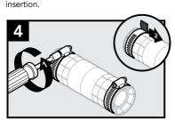
Loosen band clamps and move them towards the middle of the coupler. Lightly tighten to hold in place during conduit insertion.
