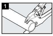
Cut conduit flush with duct cutters.
