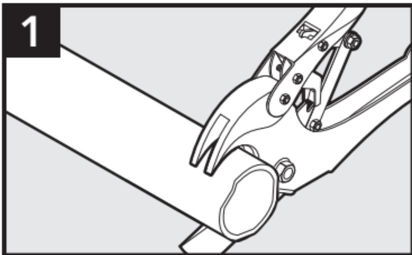
Cut conduit flush with duct cutters.
