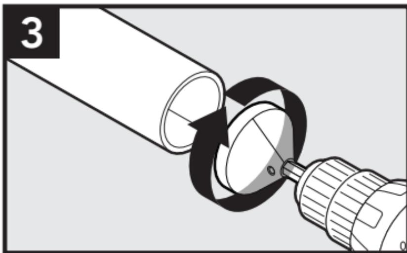
Chamfer the end to allow for smooth insertion.
