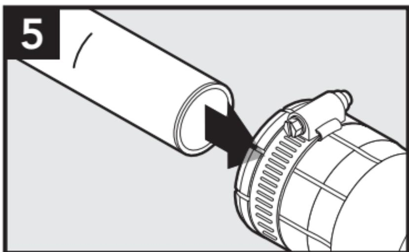
Push conduit into coupler past the metal teeth to the mark to ensure O-ring is seated around the duct.
