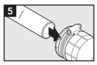
Push conduit into coupler past the metal teeth to the mark to ensure O-ring is seated around the duct.
