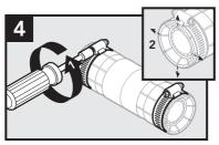
Loosen the band clamps to allow spreading of the split segments on the end of the coupler during insertion.
