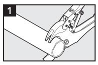
Cut conduit flush with duct cutters.
