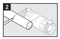
Overlap ends of conduit. Place duct at center of coupler and mark end.
